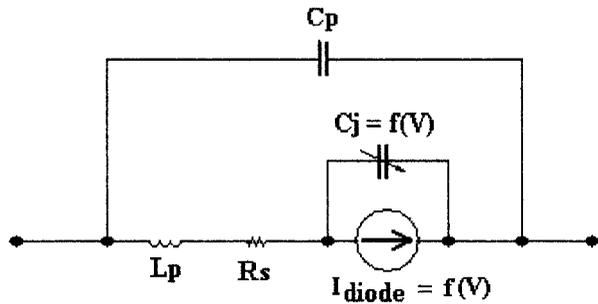
Figure 2 Nonlinear Schottky diode model
