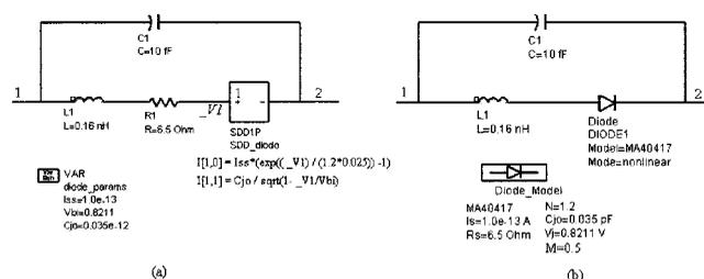
Figure 3 Nonlinear diode model for ADS using: (a) SDD; (b) diode model element
