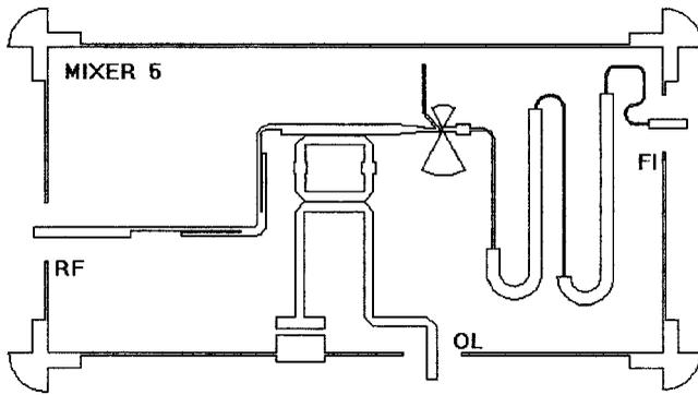
Figure 5 Layout of the X-band mixer
