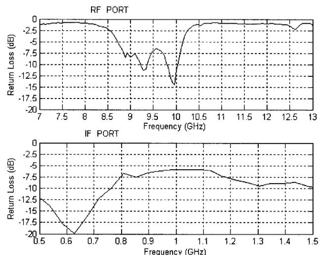
Figure 7 Return loss at RF and IF port
