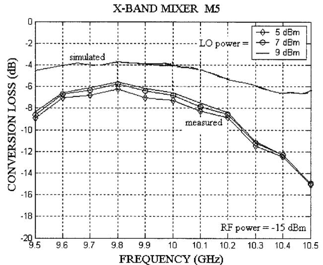
Figure 6 Frequency response of X-band mixer
