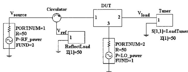
Figure 1 Load-pull simulation setup
