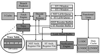
Figure 2. Trace level speculative multithreaded microarchitecture
