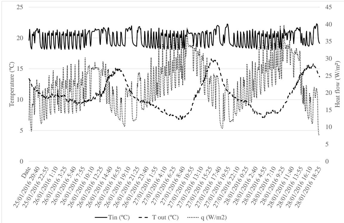
Figure 3. Data obtained from the process of monitoring Façade 2 for the period 25–28 January 2016
