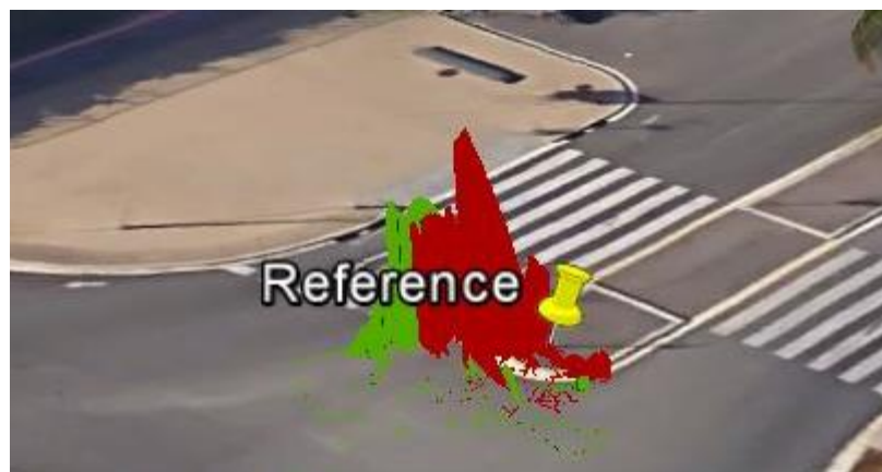
Figure 37: Test 1. NavSol - Real SVs corrected path vs. uncorrected path, horizontal path and 3D path plotted on Google Earth
