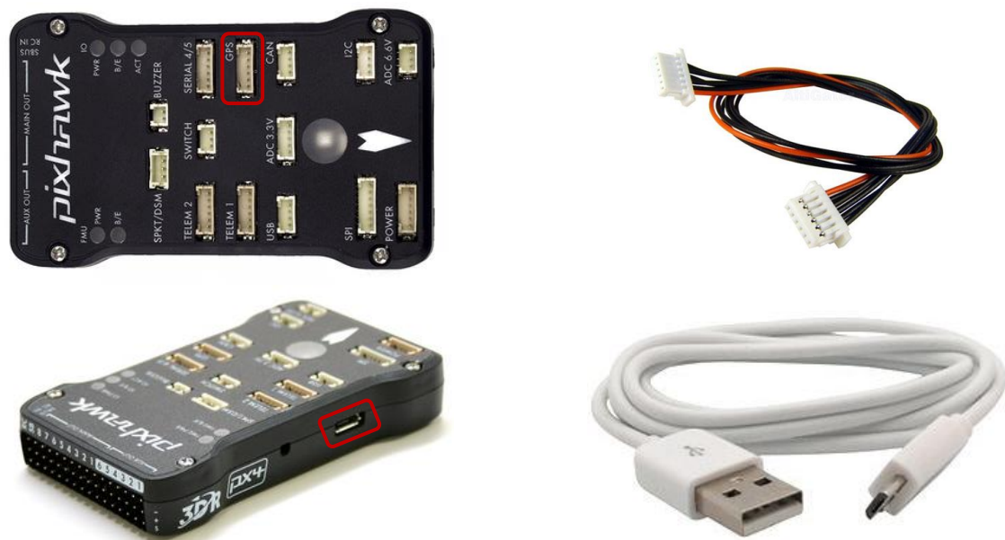
Figure 16: Pixhawk, micro USB and APM 2.5 Flight Control Cable DF13 6 Position Connector, images from https://pixhawk.org , http://mikrokopter.altigator.com/ and http://reciclatecnologia.com/ .
