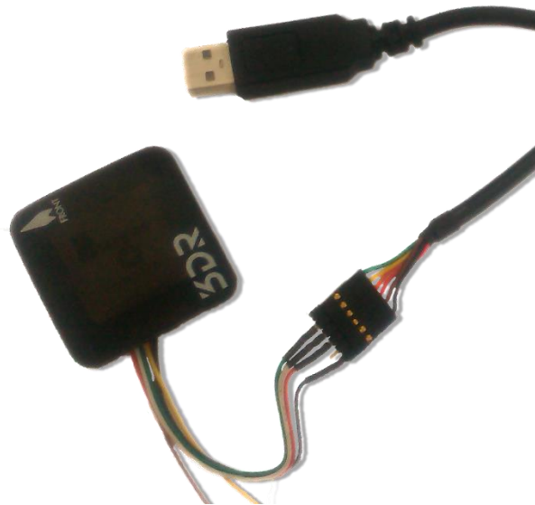
Figure 17: USB to TTL-232R serial cable to DF13 6-pin joint
