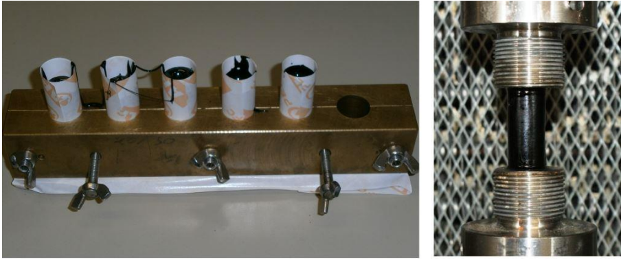
208 Figure 2. (a) Preparation of mastic specimens and (b) EBADE test set up
