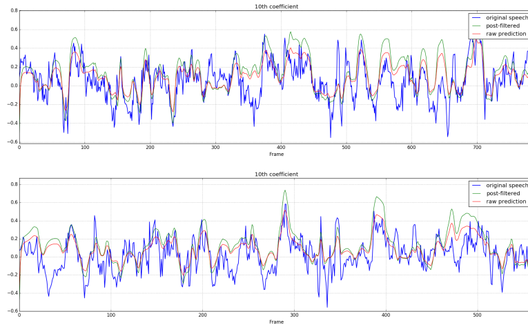
FIGURE 4.19: Evolution in time of the 10th cepstral coefficient for two test files. Blue: natural speech. Green: post-filtered prediction. Red: raw prediction.
