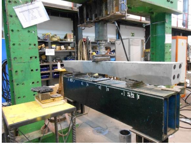
Fig. 5. Test arrangements at the centre section for the negative.
