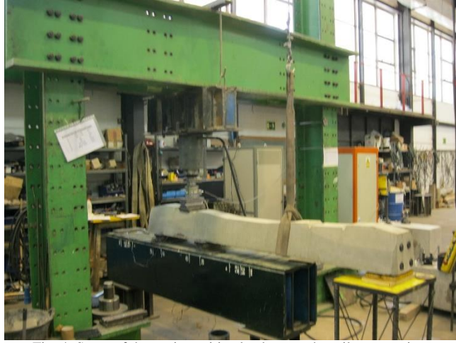
Fig. 4. Setup of the static positive load test at the rail-seat section.
