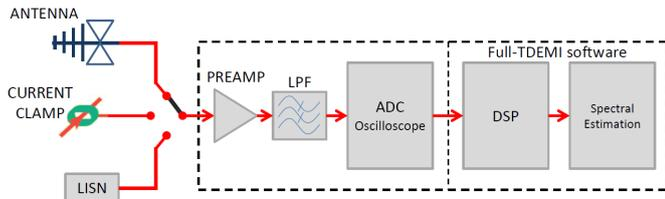
Fig. 1. Full TDEMI measurement system block diagram
