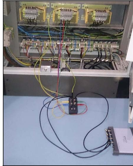
Fig. 2. In-situ example measurement for conducted emissions employing the time-domain methodology and the multi-channel in-situ voltage probe.
