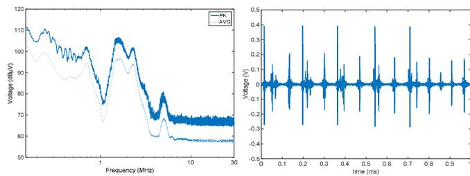
Fig. 4. Results in frequency domain with the peak and average detector and the time domain data when the rollers were measured.
