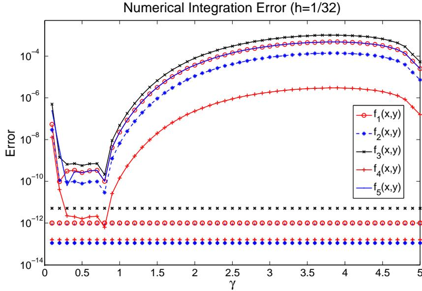
Figure 2: Numerical integration error for the Equations (5)–(9) when the parameter  $\gamma$  varies in the range  $[0.1, 5]$ . The horizontal curves (without lines) correspond to the Gauss-Legendre cubature, while the others are obtained by the approximation based on Gauss-Hermite cubature. It was used a structured mesh of hexagonal elements with  $h = 1/32$ .
