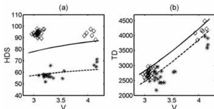
**Figure 1: Horizontal door spread HDS (m) and total drag TD (kg) as a function of towing speed V (kn). Solid line/dashed line from results of the model and diamonds/stars from experimental data (WL450/WL200 resp.).**
