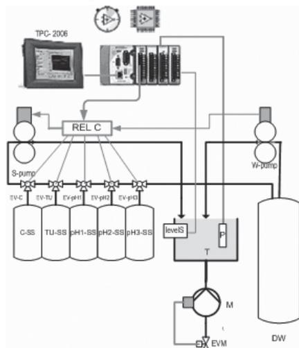
Fig. 1. WQ sensor calibration system block diagram:
