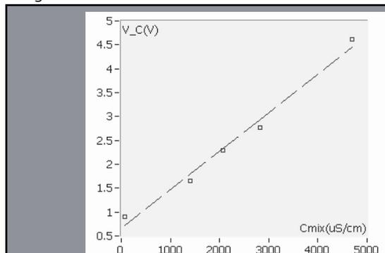
Fig. 2. Calibration curve for WQ301 sensor at 25°C.
