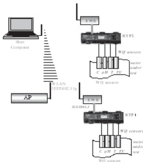
Figure 1. Distributed Measurement Systems for Water Quality Monitoring based on real-time processing unit and IEEE 802.3 and IEEE 802.1g communication protocols (AP-access point E WB-wireless bridge)
