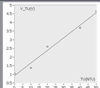
Fig 3. The WQ770 turbidity sensor calibration curve for a set of 5 calibration formazine solutions
