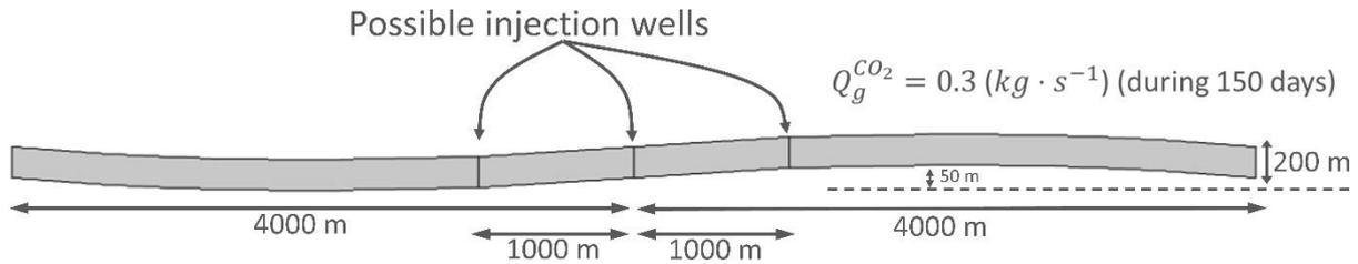
**Figure 1** Sketch of the reservoir structure targeted for the storage of supercritical CO<sub>2</sub>: 3 different potential locations of injection wells were evaluated by using numerical simulations.
