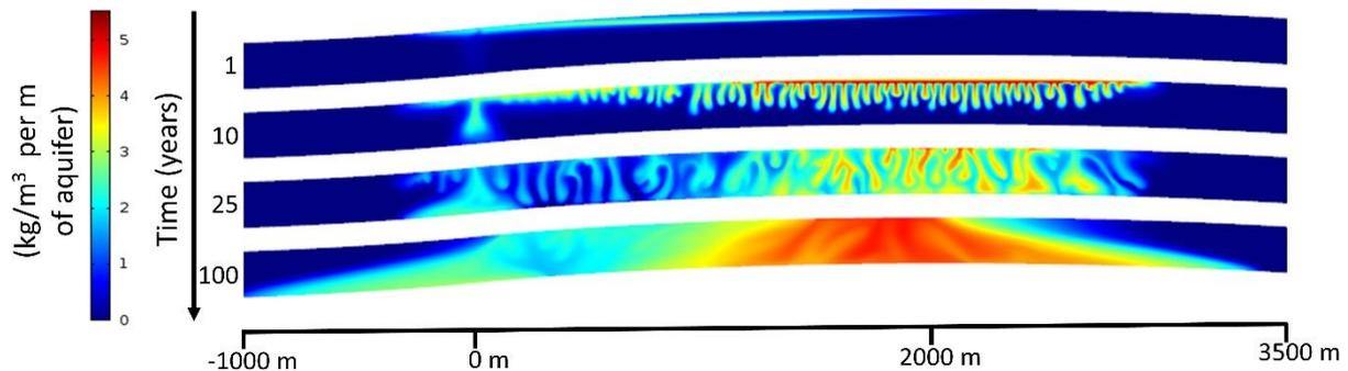
**Figure 3** 4D evolution of the CO<sub>2</sub> trapped by dissolution in the resident groundwater brine. The results correspond to the simulation for the well in the intermediate location (see Figure 2).
