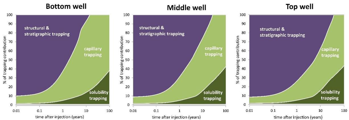
**Figure 4** Time evolution of the trapping mechanisms for the 3 different injection points.
