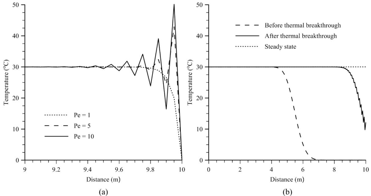
**Figure 1 (a) Temperature distribution for analyses with fixed temperature boundary condition and different values of Péclet number; (b) temperature distribution for analysis with coupled thermo-hydraulic boundary condition and Péclet number of 60**
