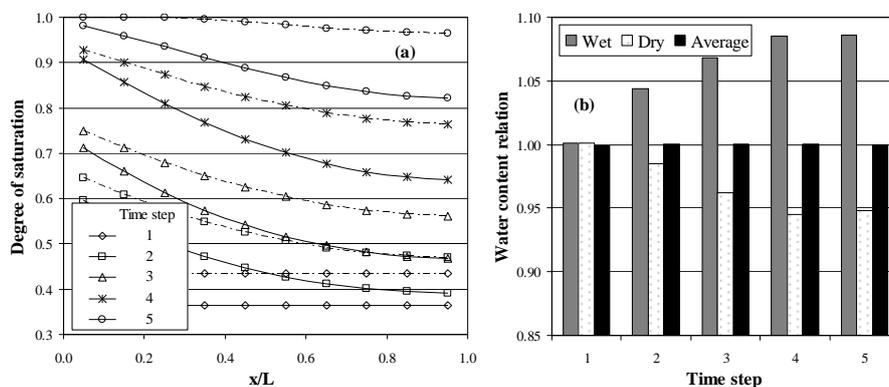
**Figure 3.** (a) Evolution of the degree of saturation at different times and for each case considered; continuous lines correspond to Case 1 and dotted lines to Case 2; (b) temporal evolution of the relation between values of water content at the wet side or at the dry side of the sample.
