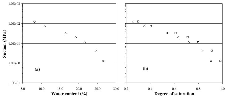
**Figure 2.** Water retention curve under constant volume conditions for a MX-80 bentonite sample compacted at a dry density of  $1.60 \text{ Mg/m}^3$ . (a) Suction against water content; (b) suction against degree of saturation.
