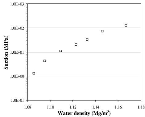
**Figure 1.** Estimated relationship between suction and average water density for a MX-80 bentonite sample compacted at a dry density of  $1.60 \text{ Mg/m}^3$ .
