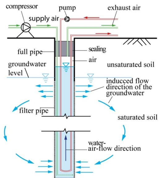
**Figure 1- air sparging borehole heat exchanger [Grabe et al. 2013]**
