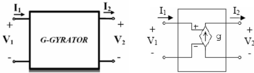
Figure 1. Basic block of a G-type power gyrator.
