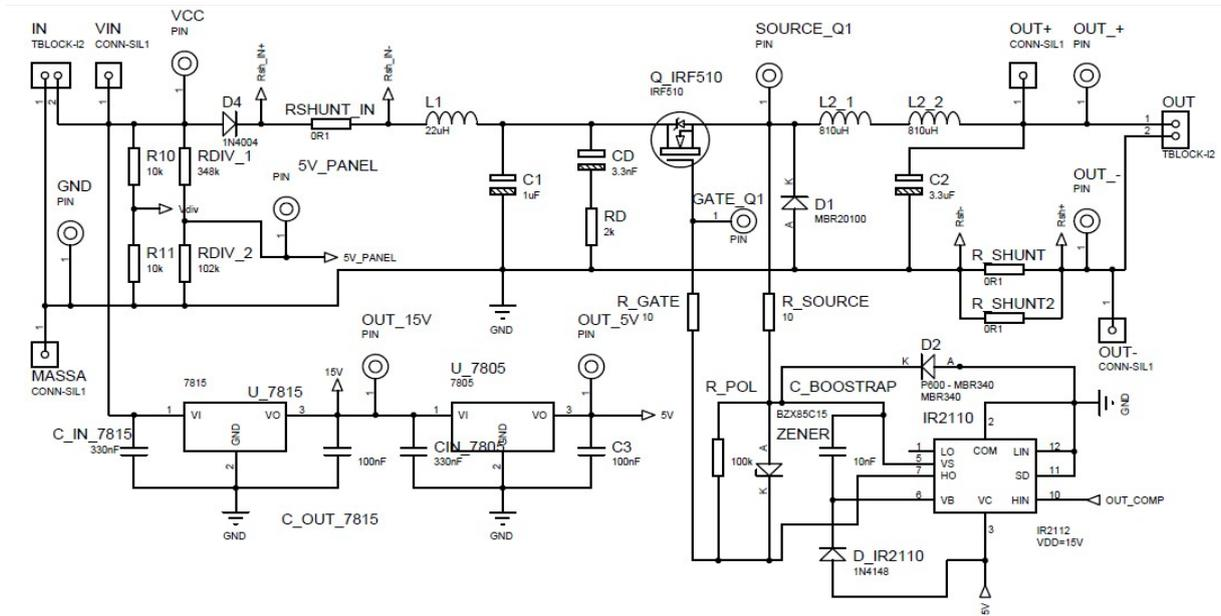
Figure 5. Schematics of the implemented BIF G-type gyrator.
