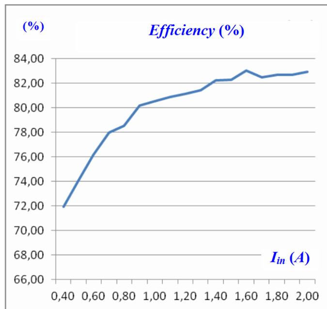
**Figure 7.** Experimental efficiency of the  $G$ -type power gyrotor for different values of the input current.
