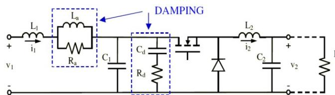
Figure 3. BIF gyrator with damping network.
