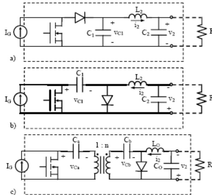
**Figure 4.** Classification of  $R$ -type gyrators: (a) boost with output filter (BOF), (b) Čuk converter, and (c) Čuk isolated.
