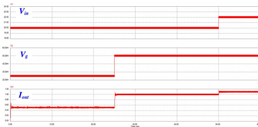
**Figure 8.** Simulation results of the implemented  $G$ -type power gyrotor.
