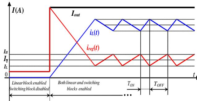
**Figure 2.** Operation principle of the proposed linear-assisted DC/DC regulator.
