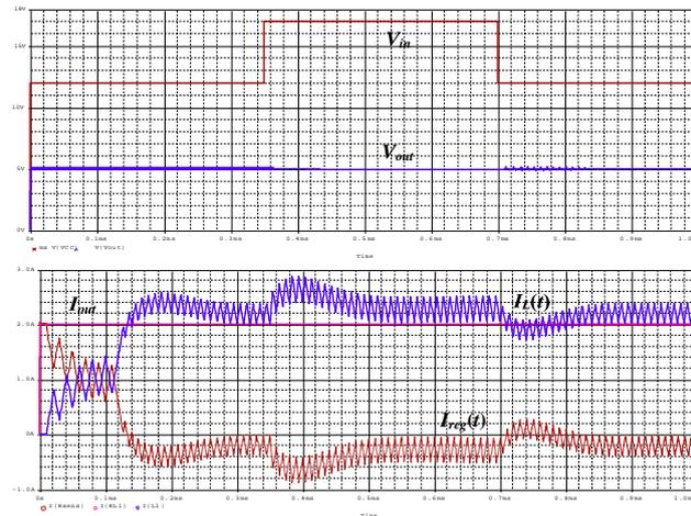
**Figure 7.** Transient response when the input voltage has an increasing step from 12 V to 17 V (variation of 41.7%) at  $t=350\ \mu\text{s}$  and vice versa at  $t=700\ \mu\text{s}$ .
