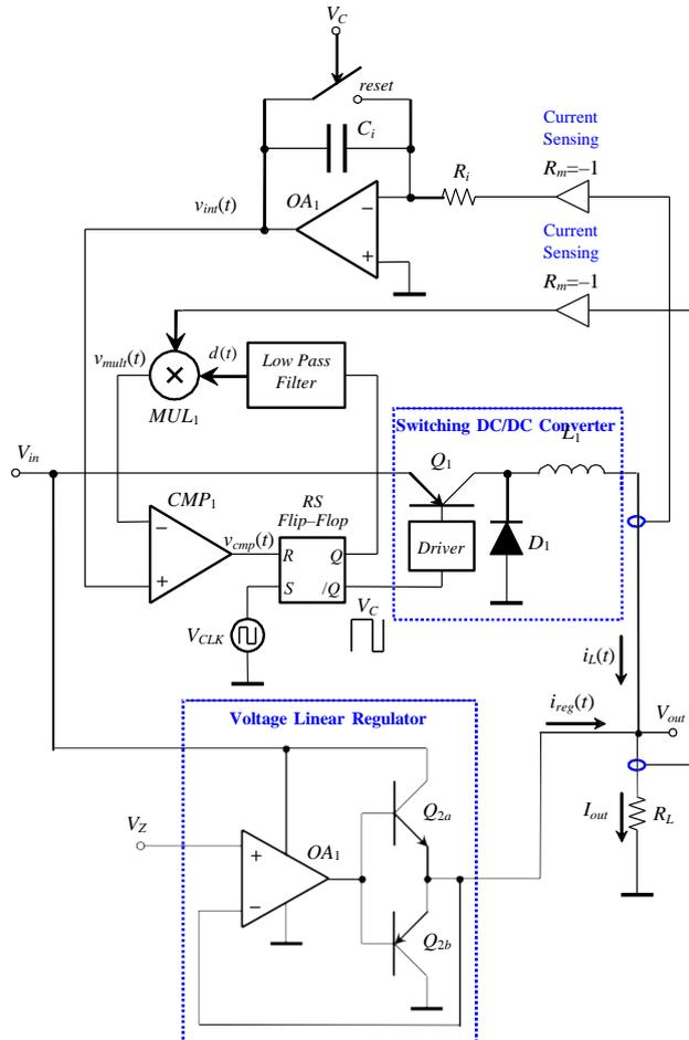
**Figure 4.** Basic structure of a modified current-mode one-cycle linear-assisted DC/DC converter.
