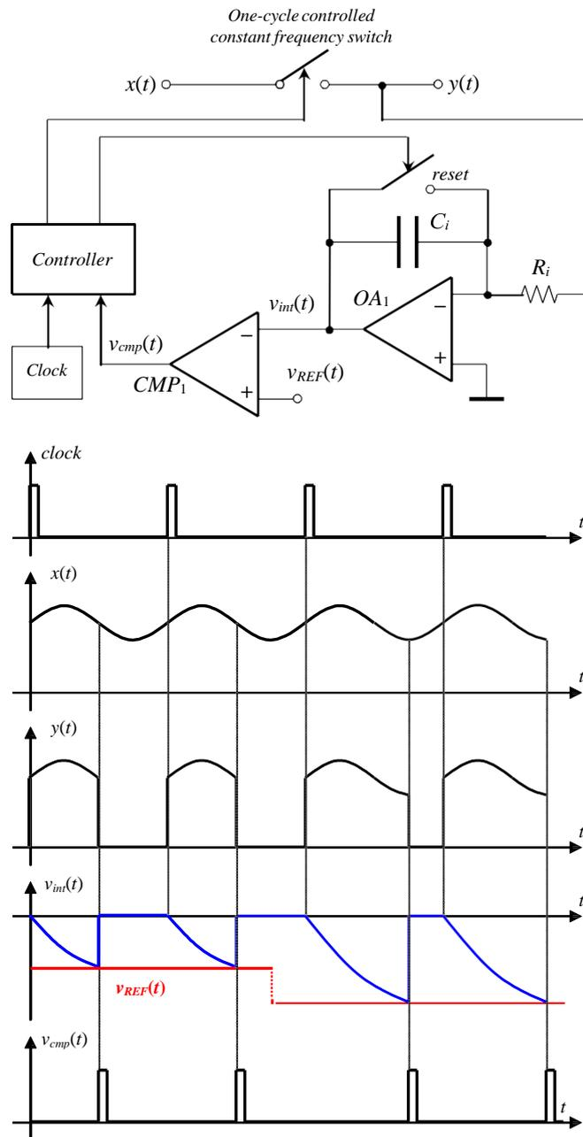
Figure 3. (a) Basic scheme of one-cycle control. (b) Typical waveforms of one-cycle control.
