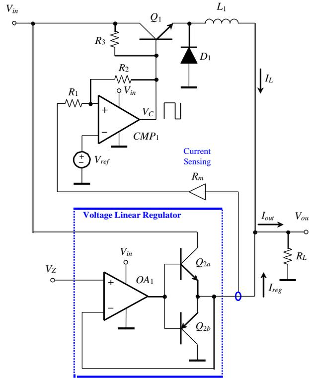
**Figure 1.** Basic structure of the proposed linear-assisted DC/DC converter.
