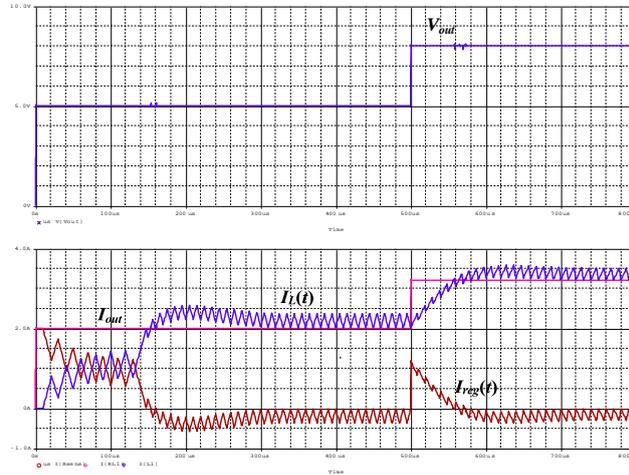
**Figure 6.** Transient response of the linear-assisted DC/DC converter to a step when the reference voltage increases from 5 V to 8 V at 500  $\mu\text{s}$ .
