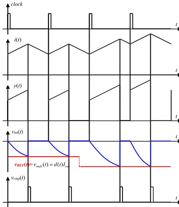
**Figure 5.** Typical waveforms of the proposed linear-assisted converter with modified current-mode one-cycle control.
