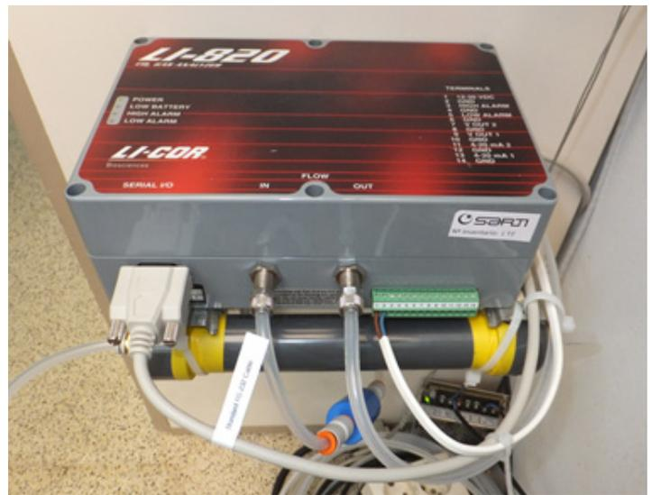
Fig 1. Atmospheric CO<sub>2</sub> measurement system
