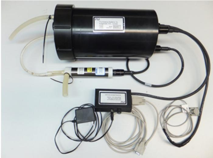
**Fig 3. Pro-Oceanus CO<sub>2</sub>-Pro CO<sub>2</sub> sensor**
