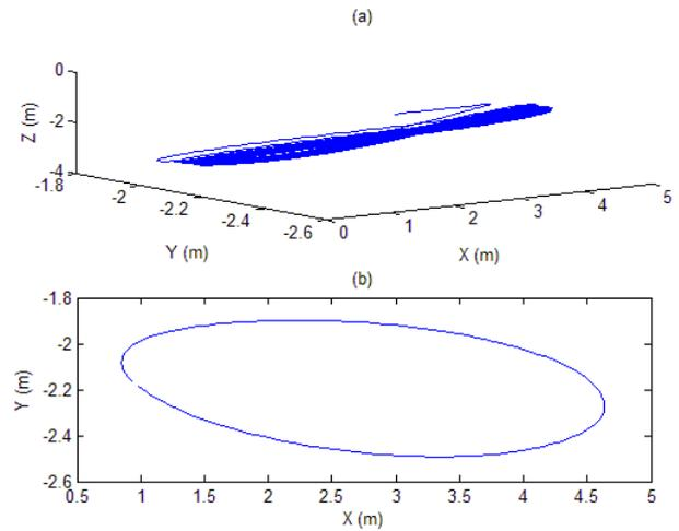
Figure 2. Buoy model. Orbit of buoy (a) from 20 s to 600 s and (b) the horizontal projection view during 1 wave period (7.52 s).
