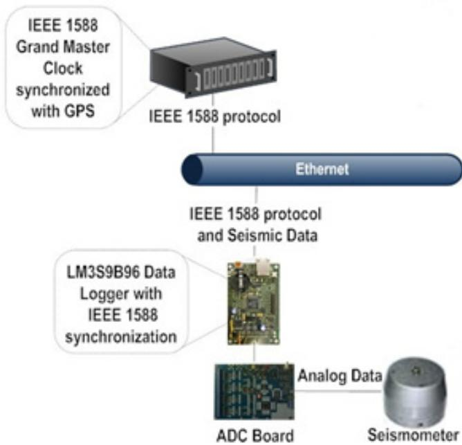
**Figure 1 Luminary LM3S9B96 Broadband Seismometer with IEEE 1588 synchronization**
