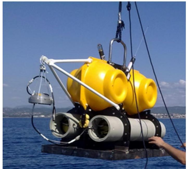
Photo 1 Ocean-bottom seismometer
