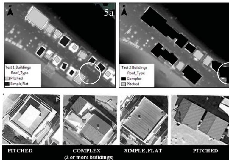
Figure 5: Visualization of types of roofs extracted. 5a) Classification of building roofs on Test 1; 5b) Classification of building roofs on Test 2; and 5c) Classification of roof types.
