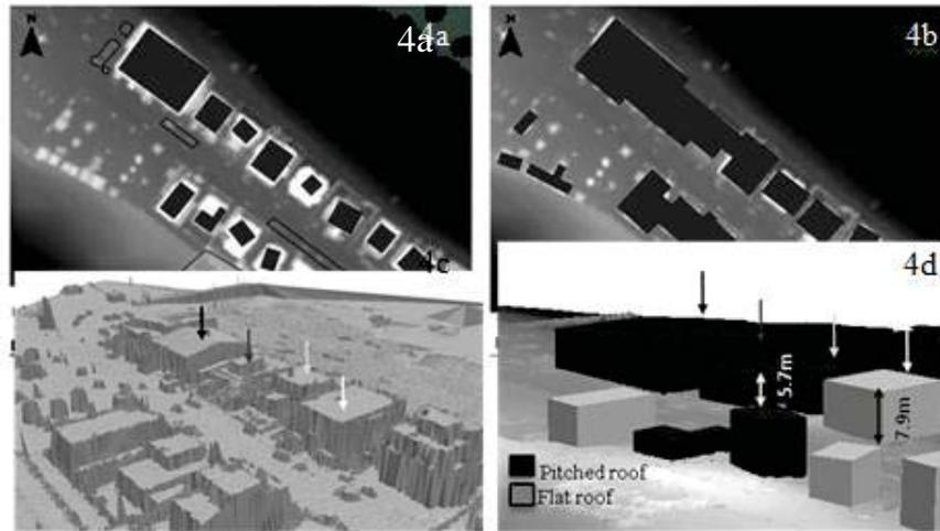
Figure 4: Visualization of buildings extracted from Test 1 and Test 2. 4a) Buildings extracted by default and polygons that identified the objects removed in Test 2; 4b) Buildings extracted by Test 2 with Refine DSM; 4c) TIN (Triangulated Irregular Network) model from LiDAR data; and 4d) 3D model buildings of Test 1.
