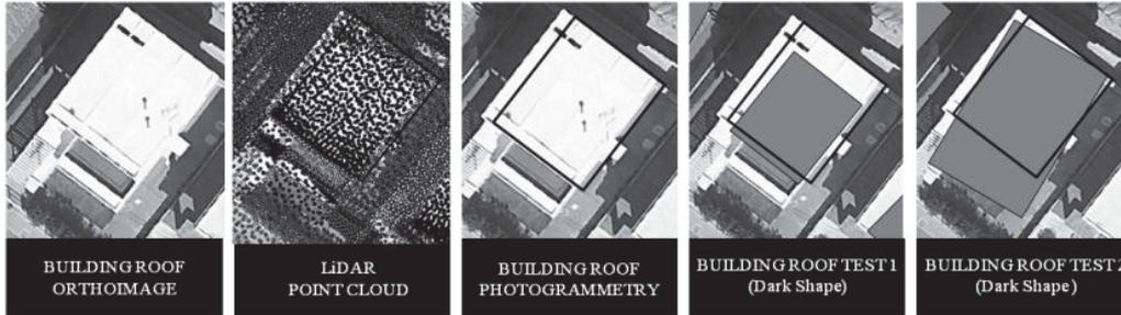
Figure 6: Comparison between the building roofs extracted by stereorestitution and LiDAR data. Influence of the building roofs extracted in the classification of roof types.
