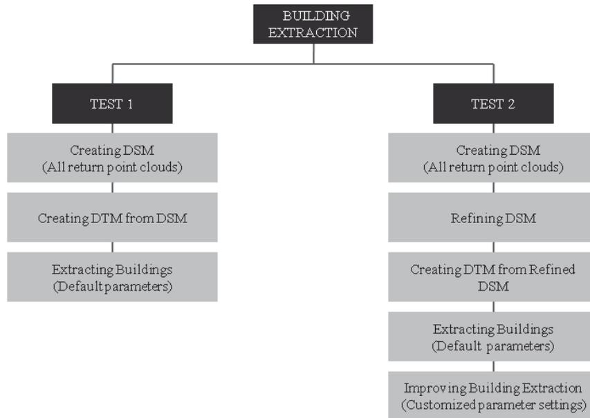
Figure 3: Two methodological approaches for building extraction based on LiDAR point cloud.
