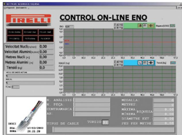
*Operator's front-end display, it allows us to verify the correct functioning of the equipments which configure the system and provides information about the parameters: velocity (m/s) and length (m) of the nucleus and aluminium and tension.*
