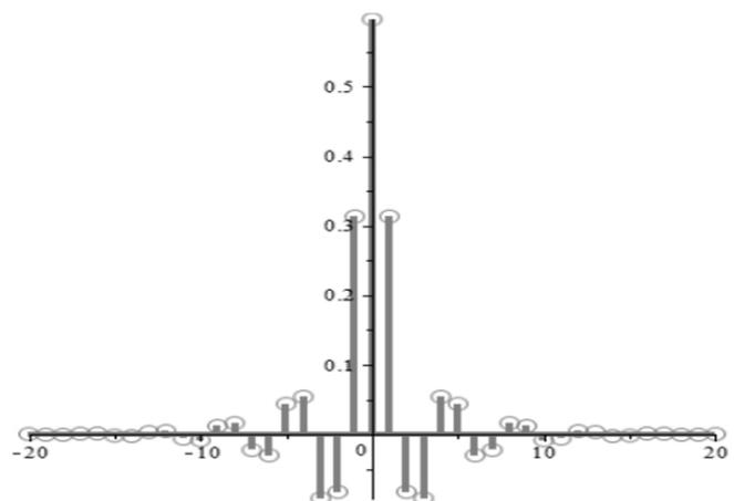
**FIR approximation of the least squares filter FIR, using 20 coefficients.**
