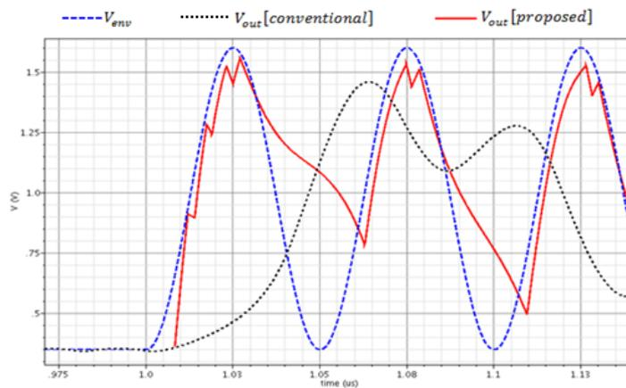
*Figure 7. Modulator's output voltage for a 20 MHz signal.*
