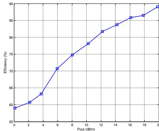
Figure 8. Plot of the efficiency of supply modulator vs. output power.
