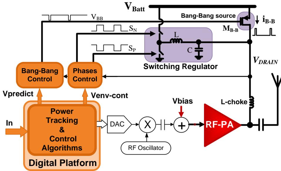
Figure 1. Block diagram of the transmitter front-end with the proposed supply modulator employing a ‘bang-bang’ slew enhancer.
