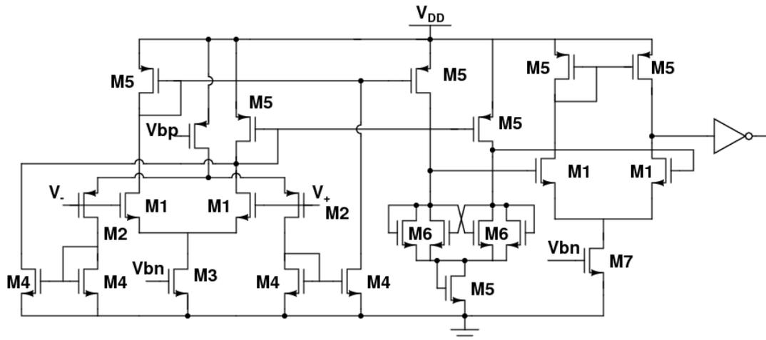
Figure 4. Simplified schematic of the comparator.
