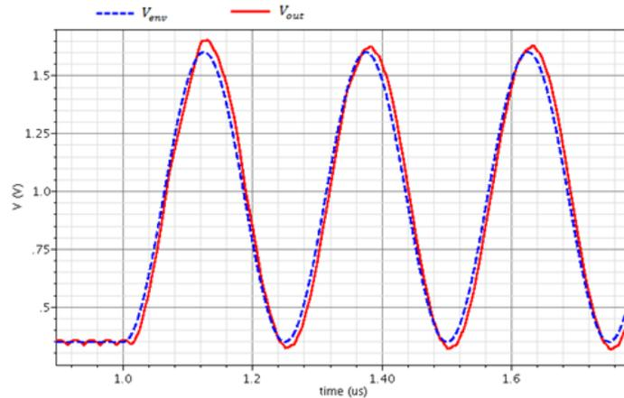
*Figure 6. Modulator's output for a 4 MHz signal.*
