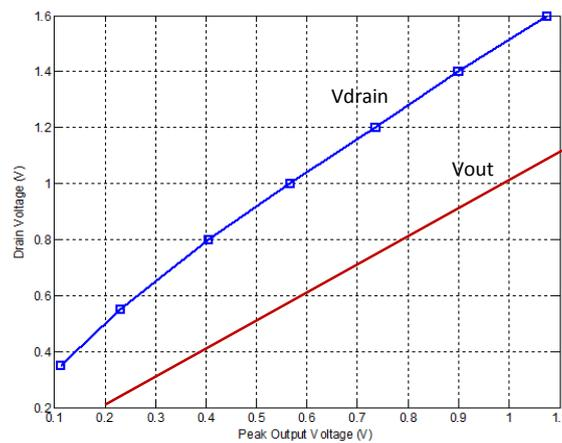
Figure 5. Plot of PA drain voltage against peak output voltage.
