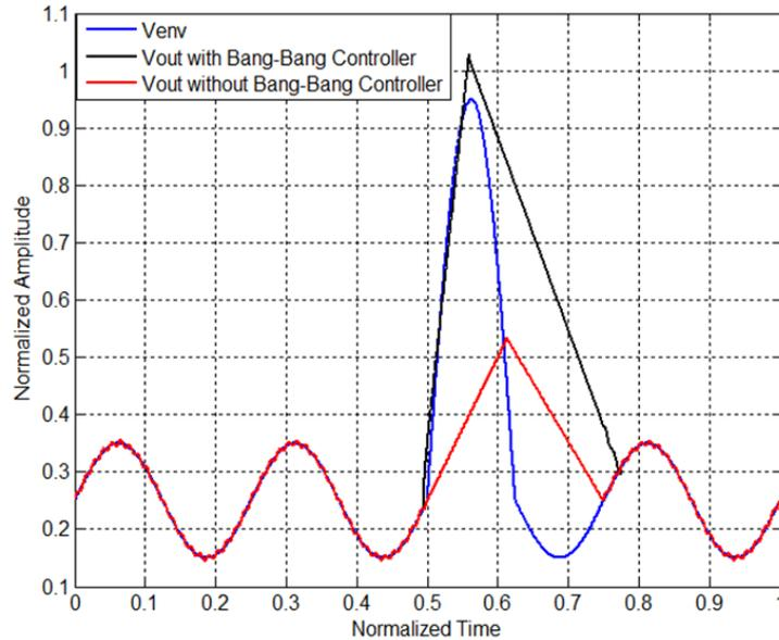
**Figure 3.** Envelope signal and switching regulator’s output voltage with and without the ideal bang-bang controller.
