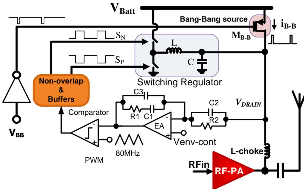
Figure 2. Circuit level implementation of the proposed architecture.
