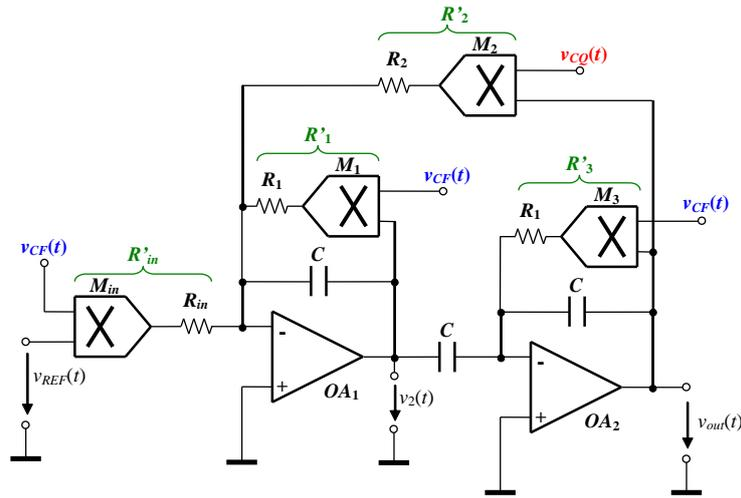
Figure 4. 2<sup>nd</sup> order analog multiplier-based band-pass filter with TQE topology.
