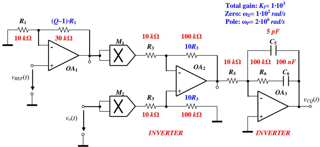
Figure 5.  $Q$ -control loop that tunes the quality factor of the CTF. The controller (operational amplifier  $OA_3$ ) acts as a pole-zero compensator.
