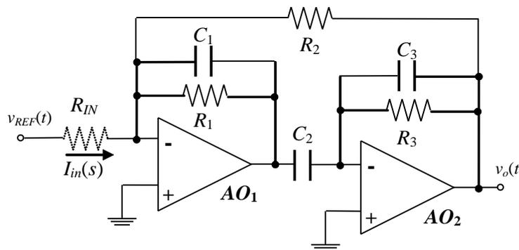
Figure 3. 2<sup>nd</sup> order band-pass filter with TQE (transimpedance  $Q$ –enhancement) topology.
