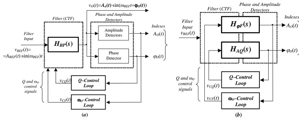
Figure 2. (a) Basic block diagram of an on-chip tuning system for a CTF. (b) CTF model with amplitude and phase detectors and control loops.
