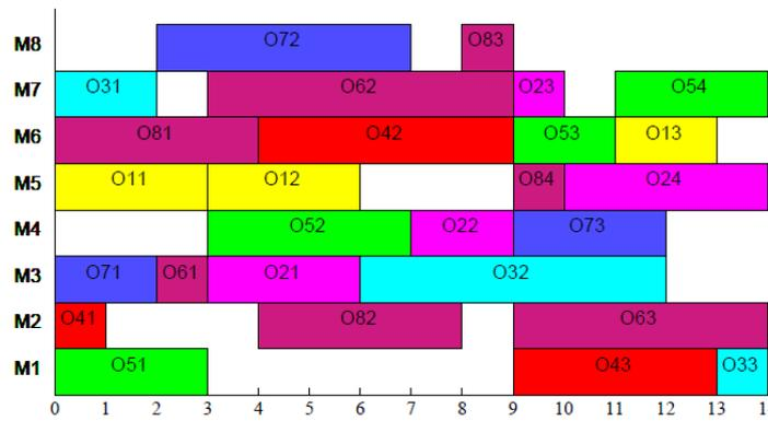
Figure 3. Gantt chart of best solution in J8M8
