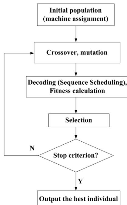
Figure 2. Flowchart of integrated GA for FJSP
