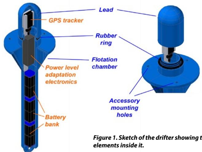
**Figure 1. Sketch of the drifter showing the elements inside it.**
