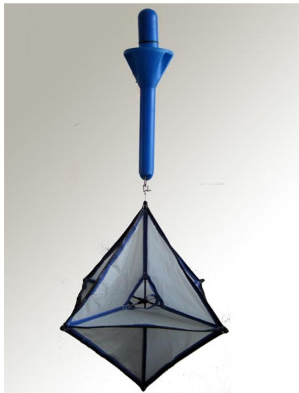
**Figure 2. Lagrangian drifter equipped with a Davis-type drogue centered at 1 m depth.**
