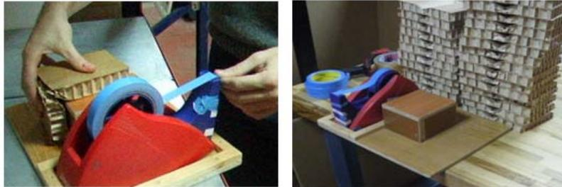
Figure 2. Poya-Yoke designed for bending protectors in WS2
