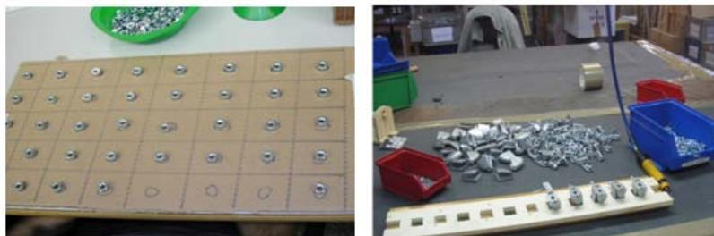
Figure 1. Poya-Yoke designed for counting parts in WS1
