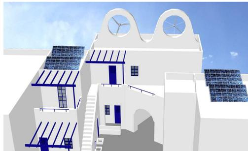
Fig. 7 Solar wind combined system on buildings of Cycladic islands
