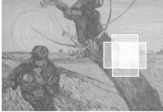
Figure 2.1: Harris Detector. A patch is shifted by a very small amount in different directions to measure local changes in auto correlation. Points, at which the correlation is large, are selected as interest points.
