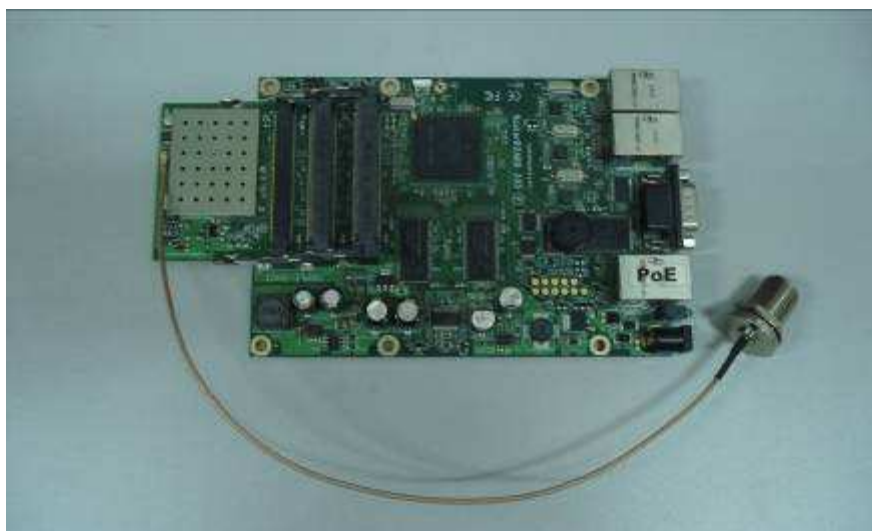
Figura 2.4: RouterBORD 333 + Tarjeta Inalámbrica R52H + pigtail
