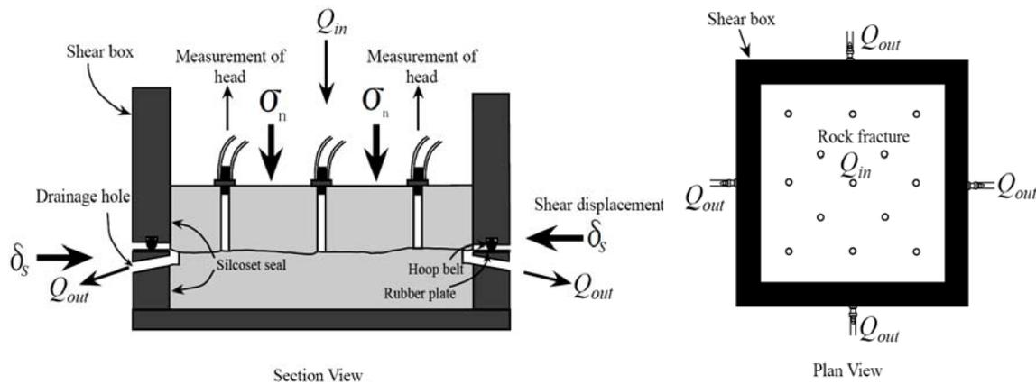
Figure 2.2. Schematic diagram of coupled translational shear-flow testing device (Yeo *et al.*, 1998). It should be noted that continuous shear loading cannot be applied in this device. The noticeable feature of this device is both radial and unidirectional flow test conditions can be considered by changing flow inlet and outlet.
