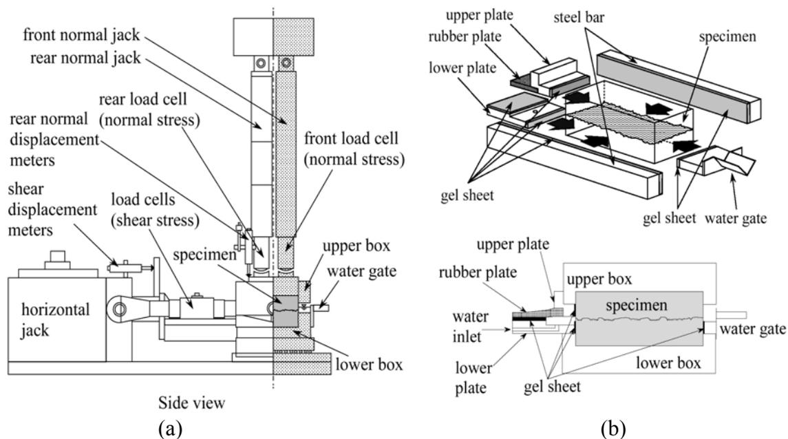
Figure 2.1. Schematic diagram of coupled translational shear-unidirectional flow testing device, (a) side view, (b) sealing mechanism of the shear box in 3D and cross section views (Mitani *et al.*, 1999). It should be noted that two normal loading jacks and cells are installed to avoid rotating/tilting of the upper surface during the tests.
