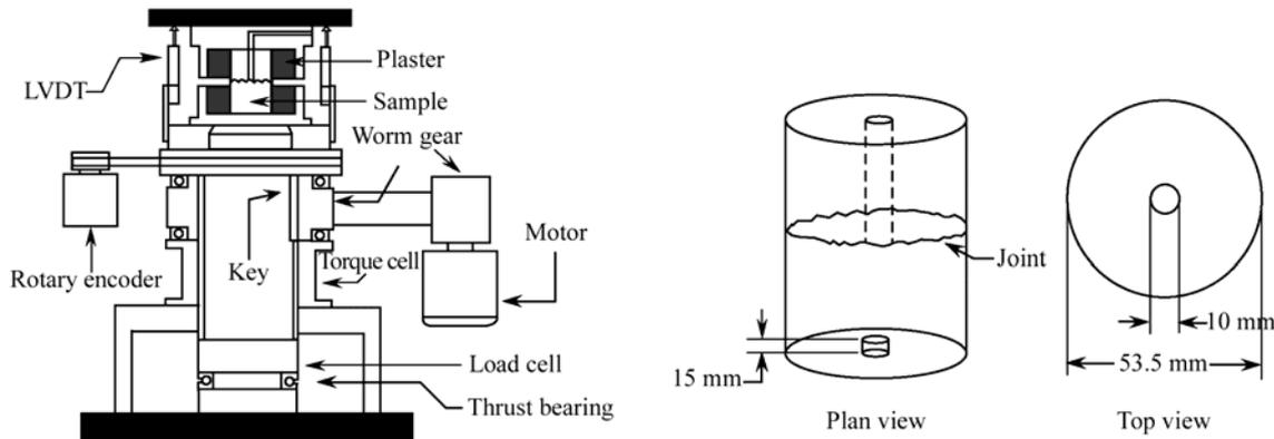
Figure 2.3. Schematic view of coupled torsional shear-radial flow testing device (Cheon *et al.*, 2002)
