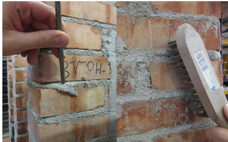
Figure 40 - The processes of cleaning the surface
