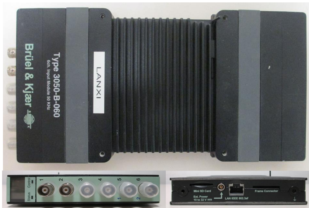
Figure 18 - Hardware of Data Acquisition System
