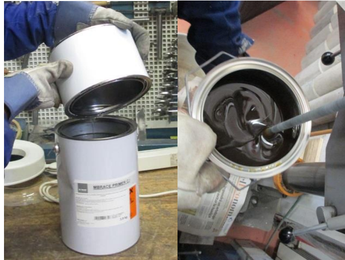
Figure 46 - Mixing the primer between 3 to 5 minutes
