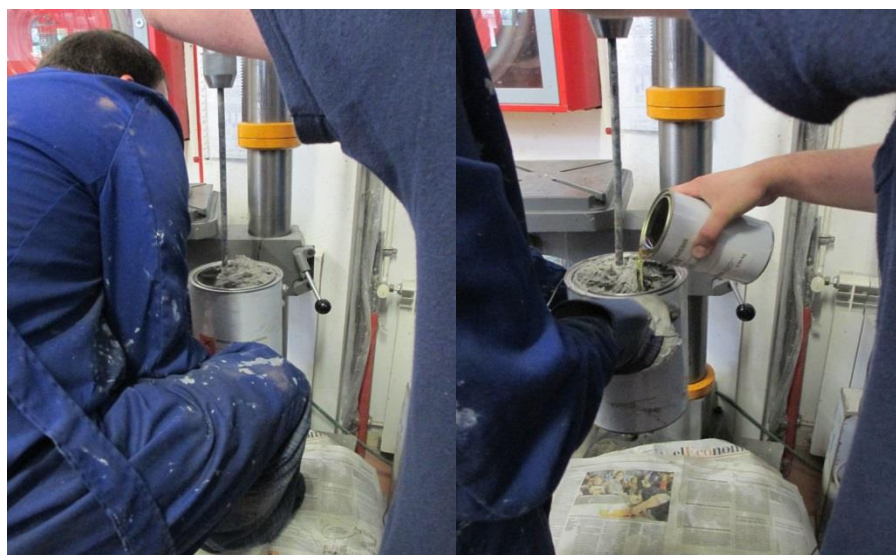
Figure 48 - Mixing and preparing the adhesive
