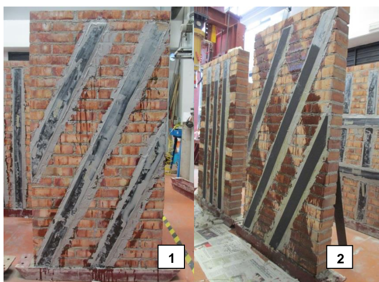
Figure 52 - Direction and turn of the second layer of FRP over the first layer of reinforcement
