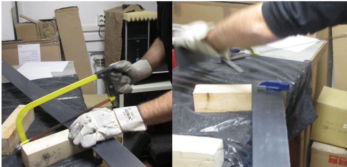
Figure 44 - How to cut the FRP
