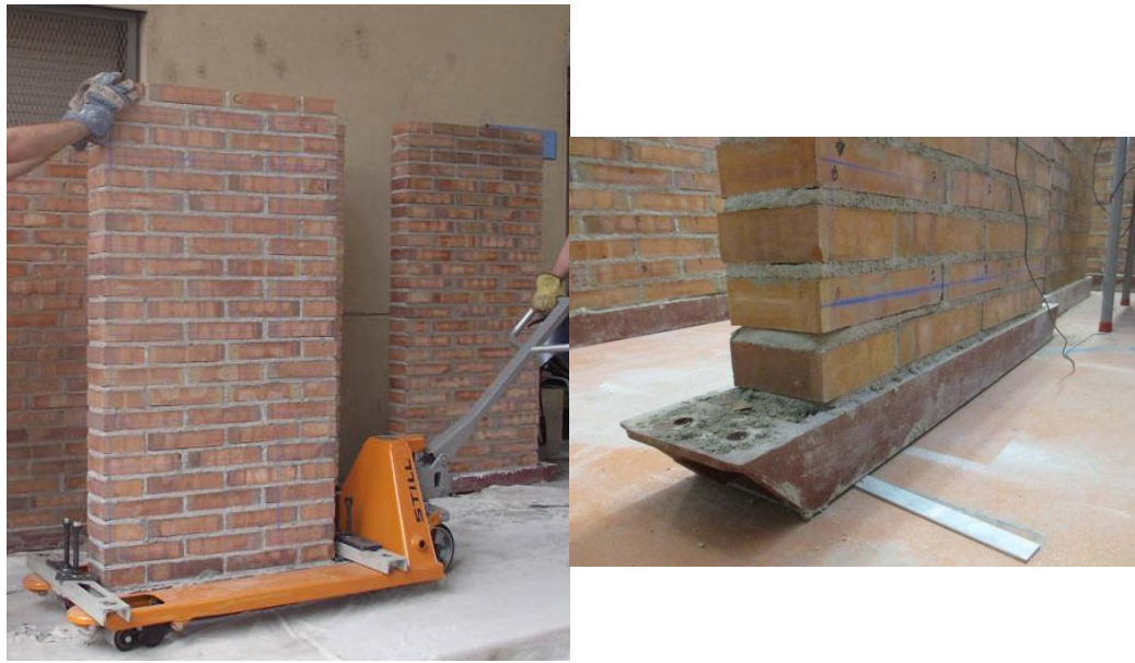
Figure 26 - Transporting and setting up the specimens in the laboratory
