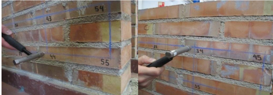
Figure 33 - Applying 2 horizontal impacts by hammer in each point
