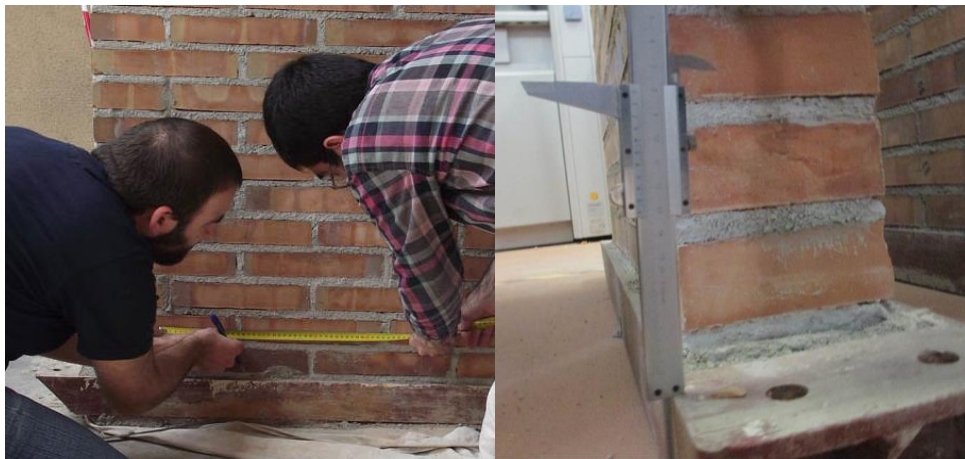
Figure 28 - Measuring the dimensions of the walls
