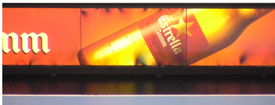
Figure 10. Detail of the stress polarization artifacts on LCDs when captured with a polarizing filter
