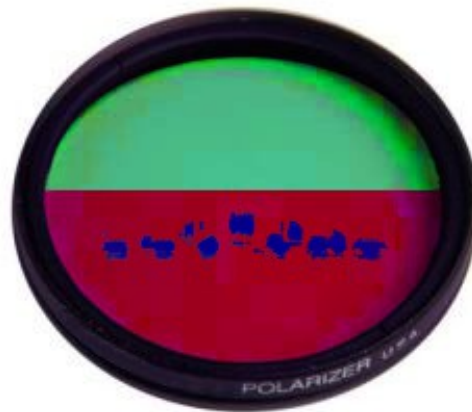
Figure 12. Pseudocolor illustrating the parts of the custom filter (green: neutral density filter, blue: linear polarizer at 0°, red: circular polarizer at 135°)
