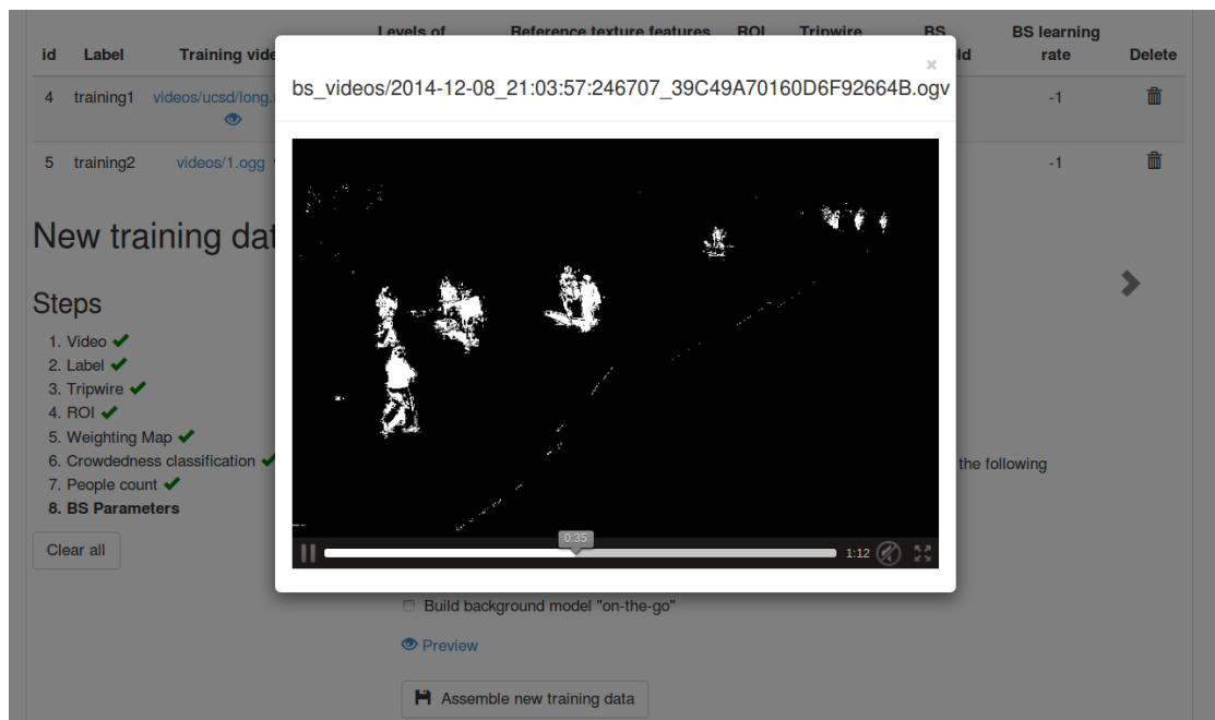
FIGURE 5.13: Web platform: new training data, BS preview. The effect of the BS parameters on the foreground segmentation can be tested using this preview feature.
