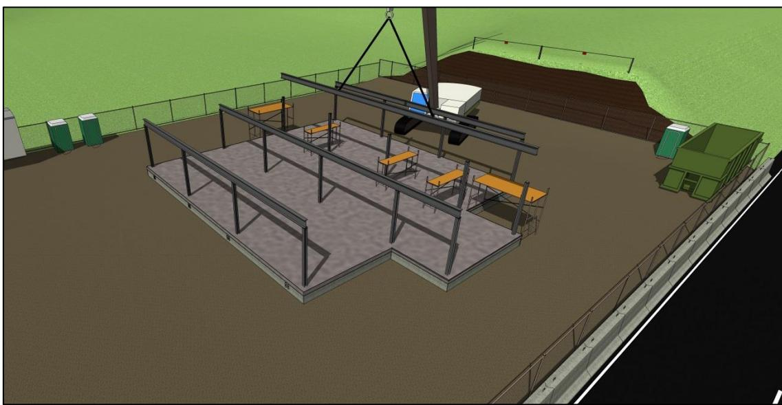
4.4 Secondary framing system
