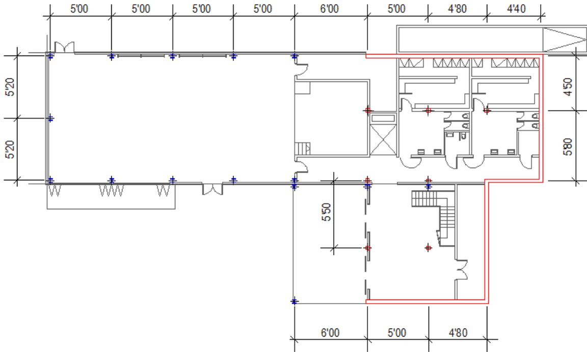
Figure 2.2: Distribution of pillars and location of the wall in the basement. PS horizontal section
