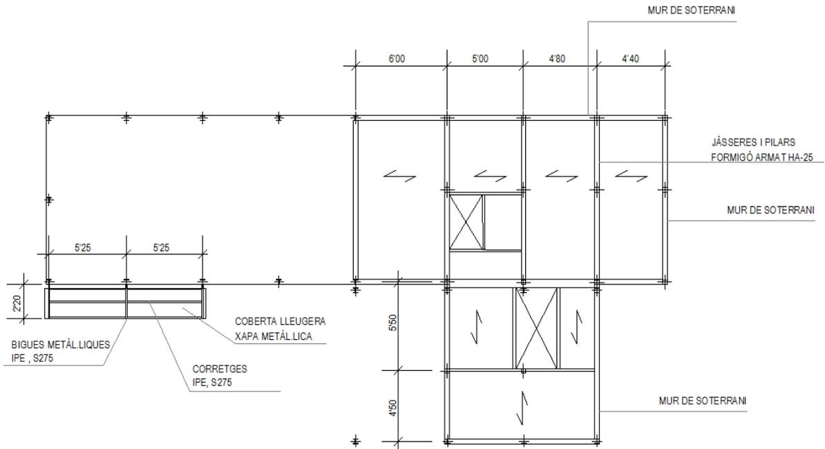
Figure 2.6: Schematic structure of the basement ceiling.
