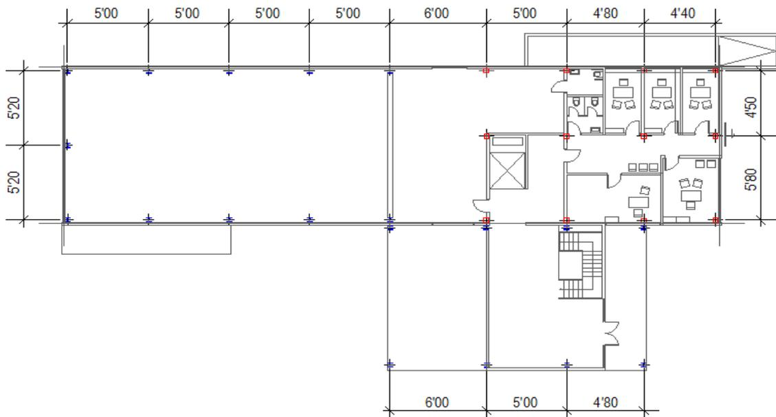
*Figure 2.1.: Distribution of pillars on the ground floor. Horizontal section PB*
