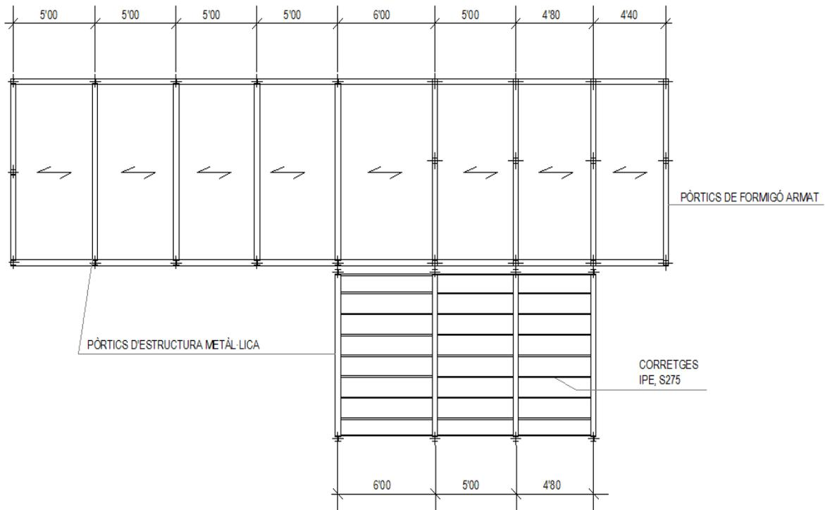
Figure 2.7: Schematic structure of the roof of the ground floor
