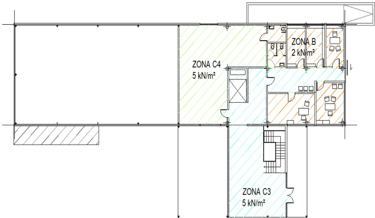
Figure 2.9: Overhead of use of ground floor roof
