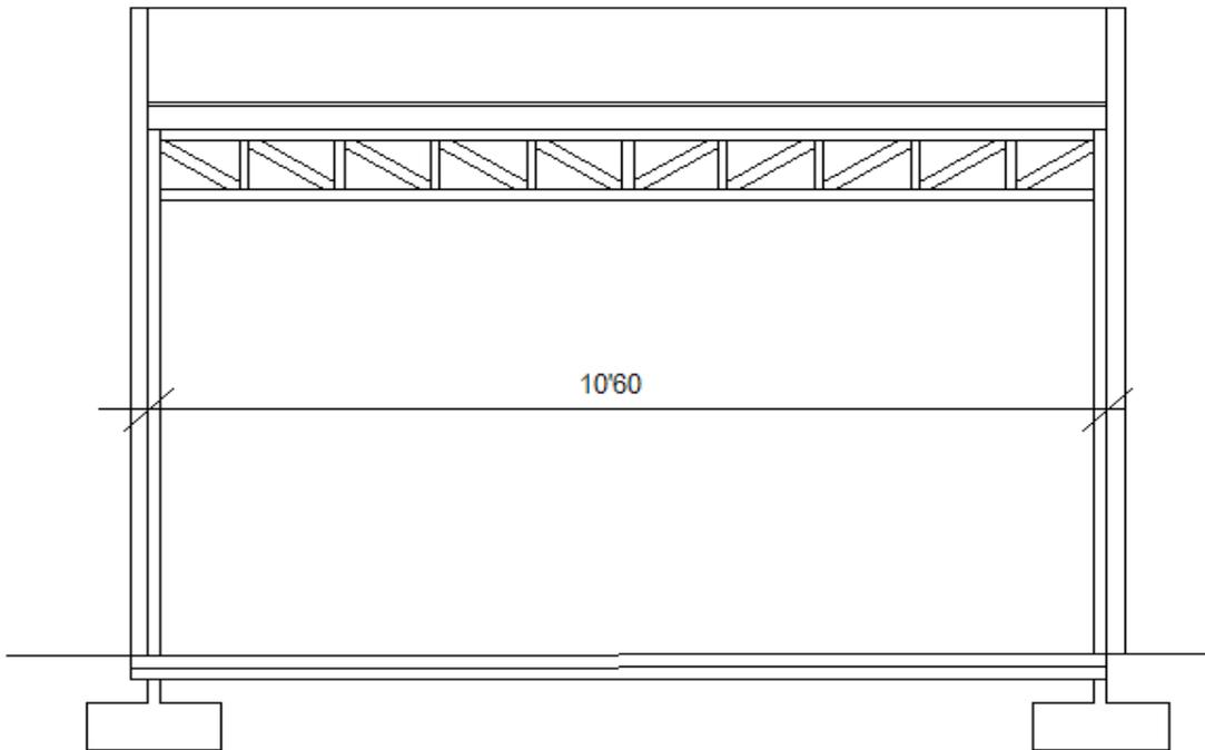
Figure 2.3: Schematic drawing of the porticos of the gym area.
