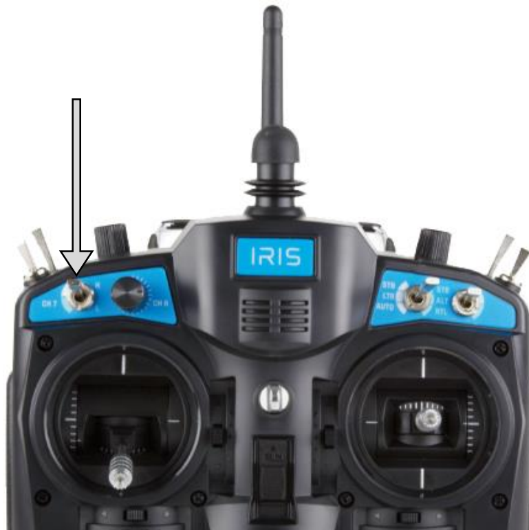
Figure 4: Manual override switch
