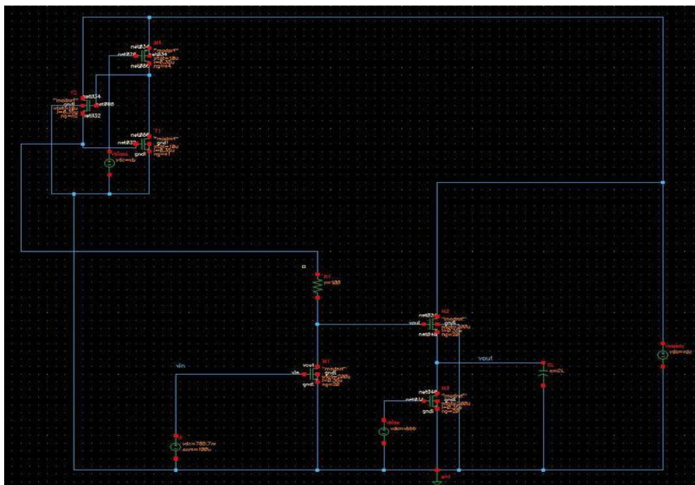
Fig. 5.2:Wideband LNA using basic active inductors
