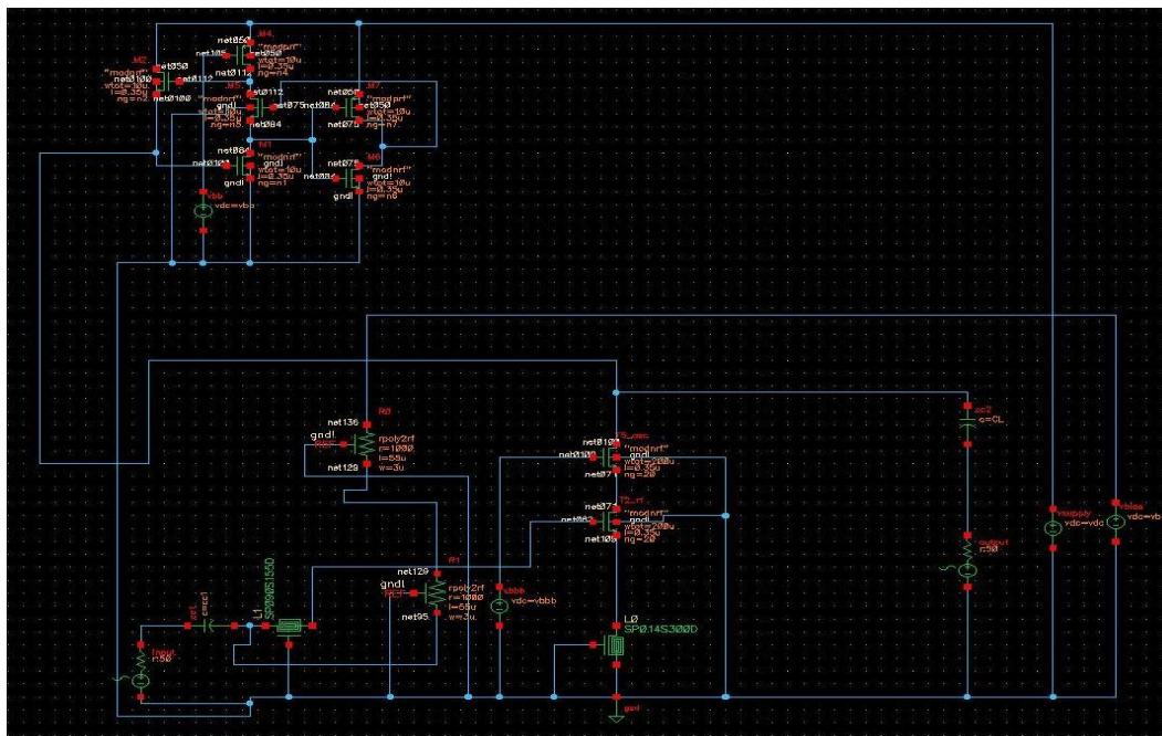
Fig. 4.8: Schematic: Tuned LNA using a regulated cascode active inductor
