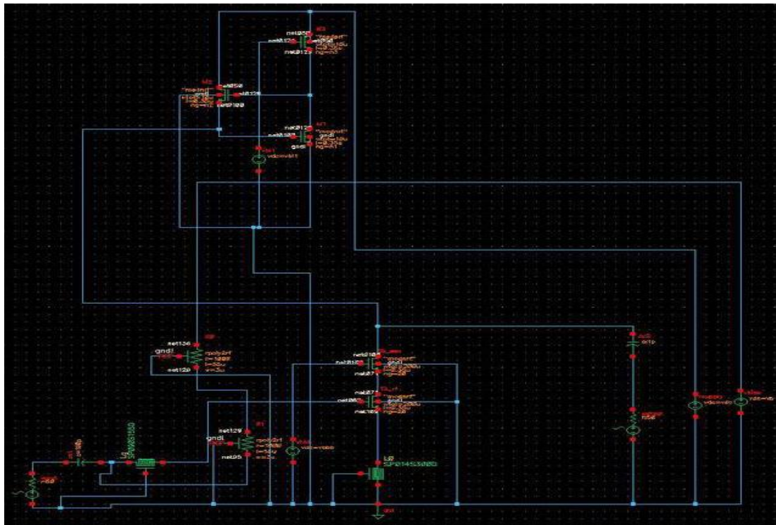
Fig. 4.5: Schematic: LNA using basic active inductor
