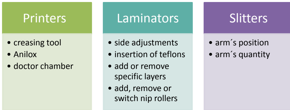
Figure 25: Changes required in the machines due to specifications changes
