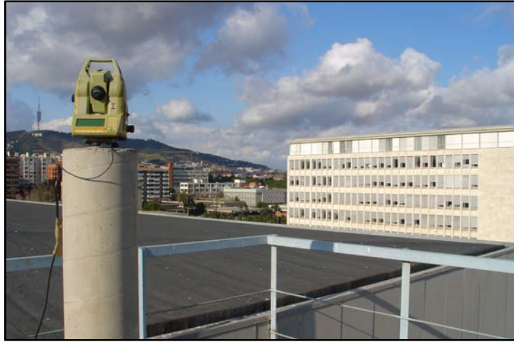
Figure 1: Structure control with AMTS (Lantada et al 2012)
