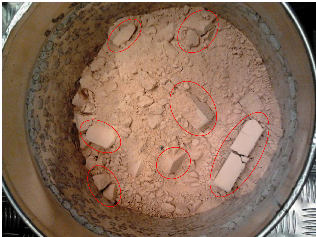
Figure 73. Raw meal tested in the uniaxial shear stress at 700 °C (big aggregates marked in red) and at lower temperatures (fine powder aggregates).
