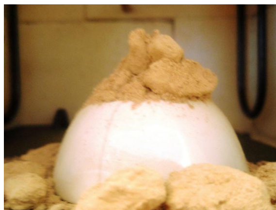
Figure 84. Performance of the angle of repose measurement at 850 °C discarded for the angle of repose measurement due to the amount of agglomerates formed.
