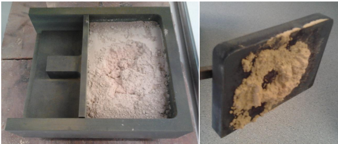
Figure 55. Removal of raw meal from the uniaxial shear test cell at 850 °C (left). Raw meal stuck to the consolidation lid at 850 °C (right).
