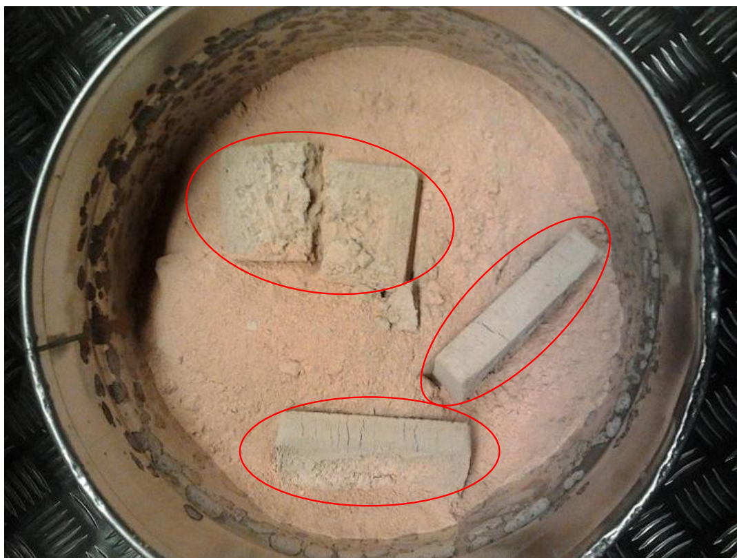
Figure 74. Raw meal tested in the uniaxial shear stress at 850 °C (huge powder blocks marked in red) and at lower temperatures (fine powder).
