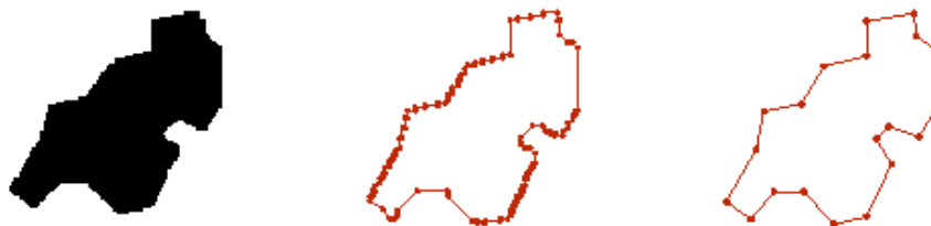
Figure 19: A polygon on the Binary Partition (Left); A high density pre-simplified polygon (Center); the final simplified polygon (Right).
