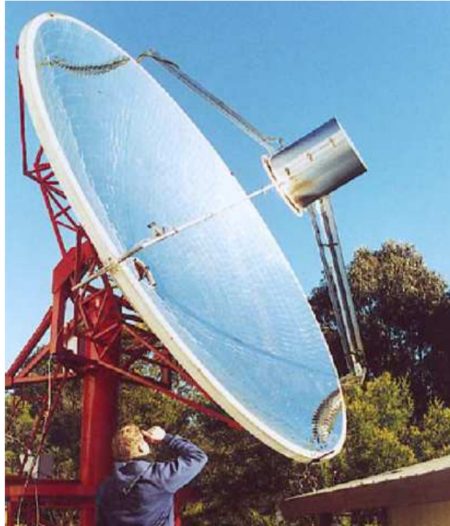
Figure 36. 15\text{ kW}_{\text{sol}} ammonia dissociation receiver/reactor in operation on the ANU 20\text{ m}^2 dish [37].
