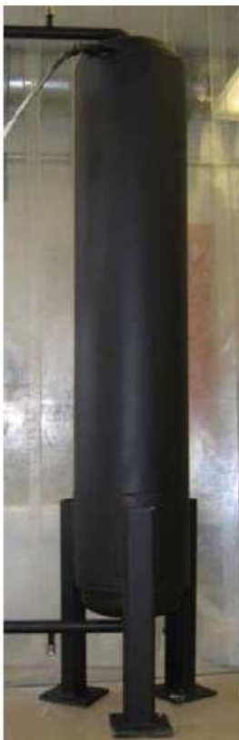
Figure 26. \text{NaNO}_3 PCM Storage Test Module [27].
