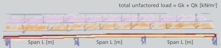
Triple-span beam for total unfactored load = G_k + Q_k for L/400 unfavourably superposed G_k/Q_k = 0.5 to 1.5
