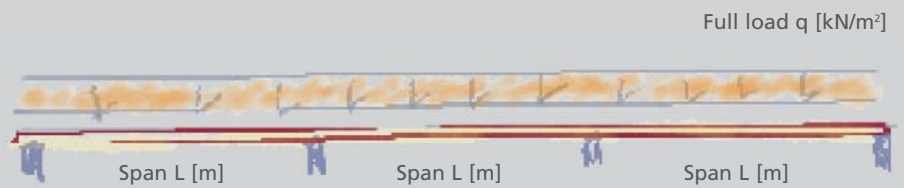
Triple-span beam for total unfactored load = Gk + Qk for L/300
