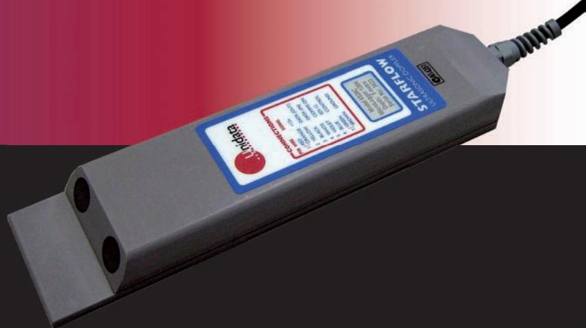
transducer assembly is profiled to reduce flow disturbance and signal electronics. It is designed to be placed at (or near) the bottom of the water channel for upstream measurement. A single cable connects the instrument to a 12V DC power source.
