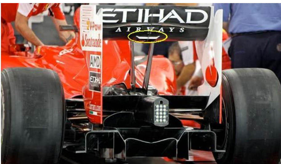
Fig. 2.42 – 2010 Ferrari F1 car [6], with the slot positioned on the central section of the main plane.
