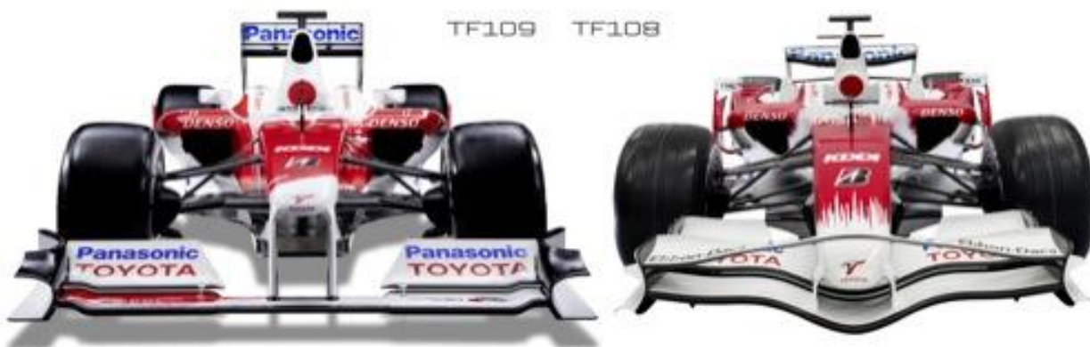
Fig. 2.88 – Toyota F1 with extremely developed shapes (right) from 2008 season, and the adaptation of the aero packaging for 2009 season (left), with completely straight profiles [10].
