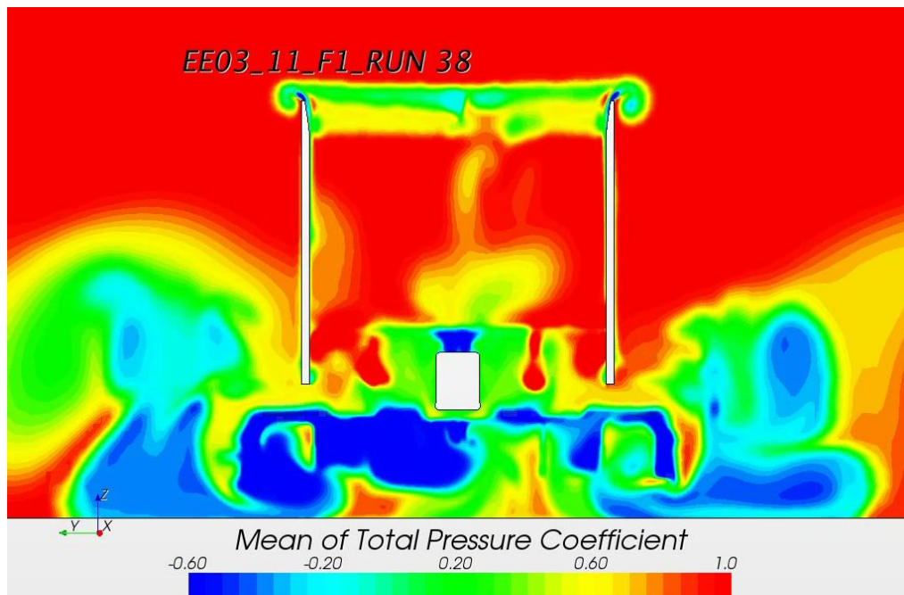
Fig 2.124 – Former rear wing wake generated at X=3610 mm from the front wheel axis. Notice the asymmetry of the flow again, especially in the diffuser area rather than the rear wing.
