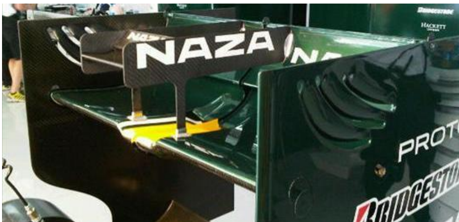
Fig. 2.41 – 2010 Lotus F1 rear wing [6], with an extra element mounted on the central section (actually, it is a 2-element wing with their own endplates, so it is clear the freedom of design in this central section).
