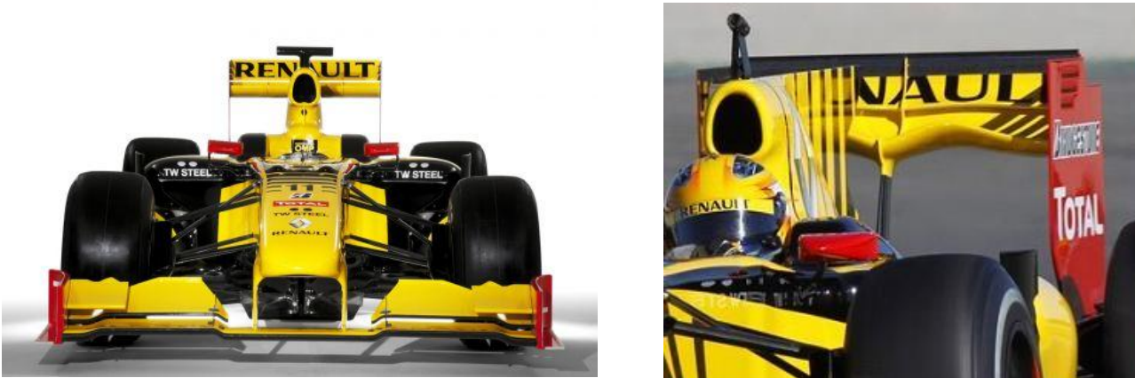
Fig 2.89 – Renault F1 2010 car launch (left) and the evolution after a few weeks of testing (right) during the winter tests in Jerez, 2010. Notice the “seagull” shape of the main plane [10].
