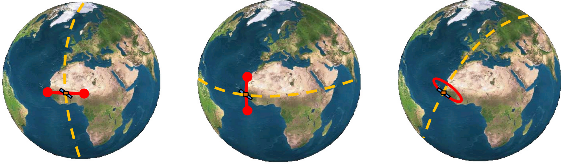
Fig. 5.13 Earth zones (yellow slashed lines) which will see the largest along-track satellite motion for different orbital configurations.
