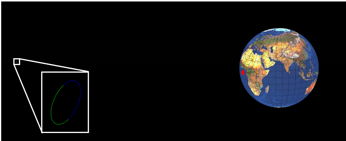
Fig. 5.11 3D satellite orbit representation considering a 0.046 degrees inclined orbit with 0.0004 eccentricity and nominal longitude of -30 degrees with respect to an Earth's centred rotating coordinate system.
