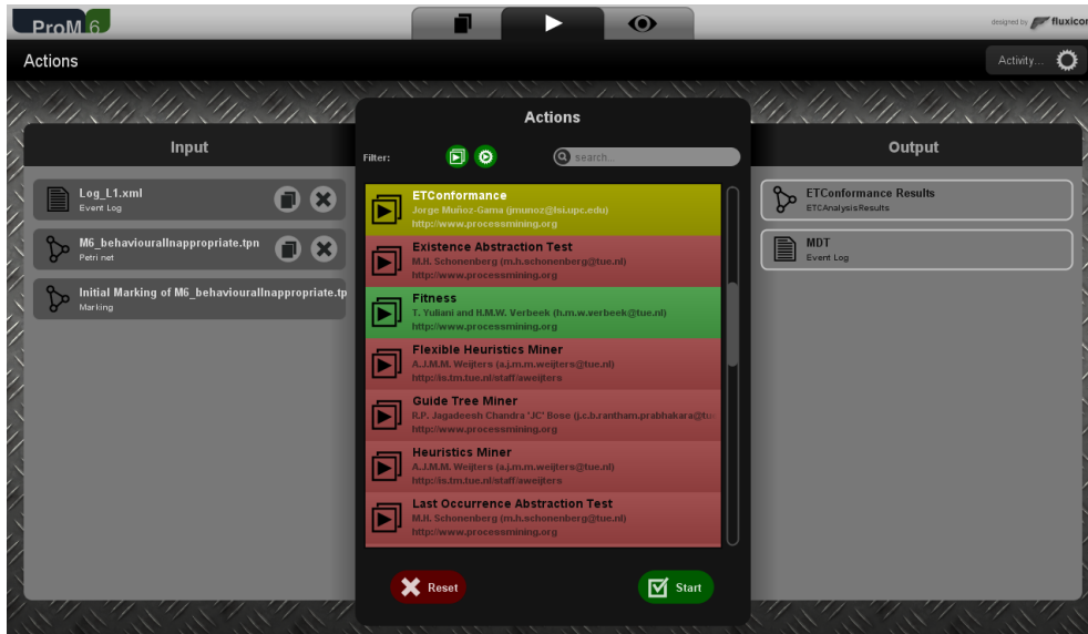
Figure 5.1: Initial Dialog of ETConformance plug-in. The plug-in requires a log, and a Petri net with its initial marking. It outputs the conformance analysis results, and the set of Minimal Disconformant Traces (MDT).
