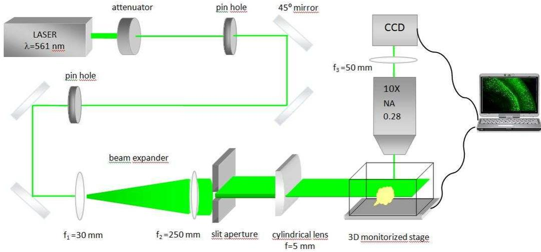
Figure 2. Ultramicroscope setup.
