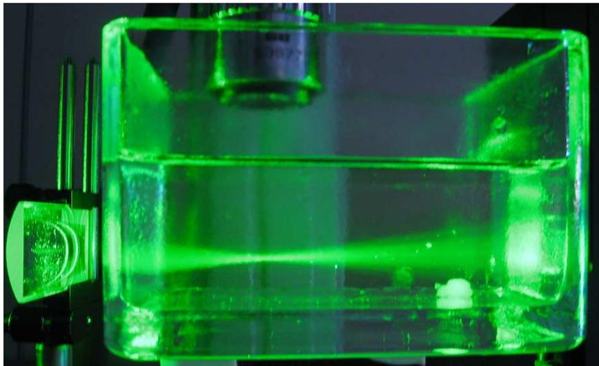
Figure 10. Example of light sheet for a slit aperture diameter of 10 mm.
