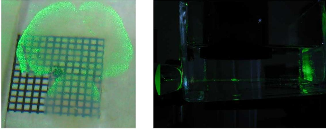
Figure 1. Optical section in a transparent sample: (a) view from the top, (b) lateral view.
