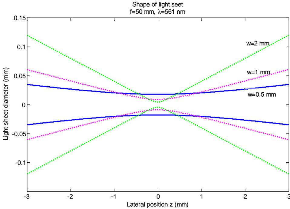
Figure 3. Lateral view of the light sheet.
